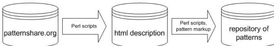
Figure 5.12: The pattern extraction process. (1) Information about the security patterns is extracted from the patternshare.org repository using Perl scripts; (2) the pattern descriptions are then converted to an XML format using Perl scripts and a pattern markup language.
