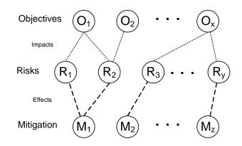
Figure 3.1: Topology of a DDP Model
