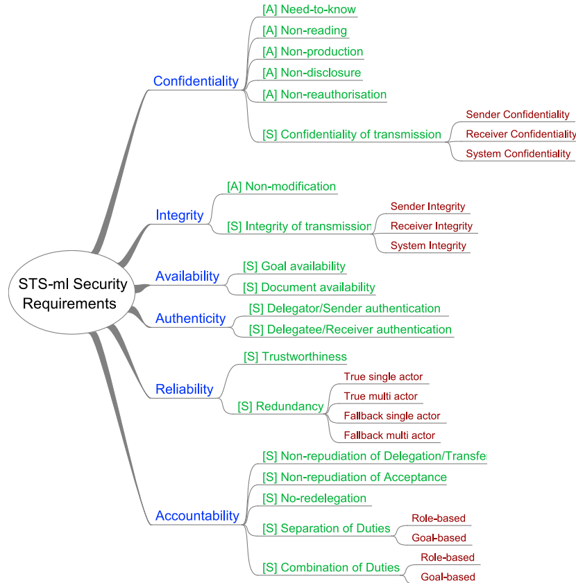
Figure 4: Security requirements types in STS-ml, classified according to information security principles, and indicating the view that enables expressing them (A=Authorisation, S=Social)
